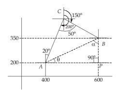
$$\angle C = 200^{\circ} - 150^{\circ} = 50^{\circ}$$
