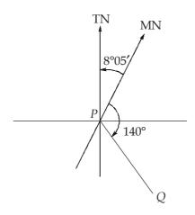
True bearing of PQ = Magnetic bearing  $\pm$  magnetic declination E/W =  $140^{\circ} + 8^{\circ}05'$  =  $148^{\circ}05'$
