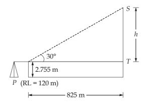
RL of top of tower = Height of instrument at
