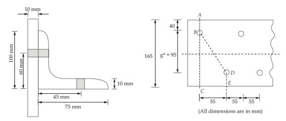
Since both legs are connected and so outstanding leg is rotated and resulting section is shown in above figure.
