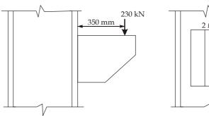
Direct shear stress,  $q = \frac{P}{2t \times d}$
