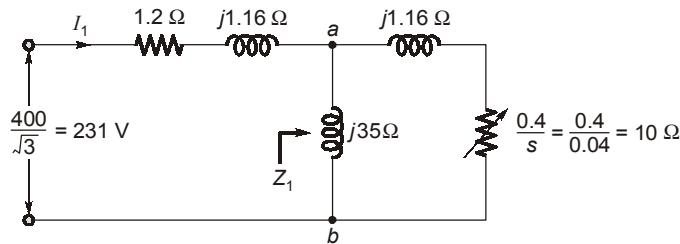
$$\begin{aligned} Z_1 &= \frac{j35(10 + j1.16)}{10 + j(35 + 1.16)} \\ &= \frac{352.45 \angle 96.6^\circ}{37.51 \angle 74.5^\circ} = 9.4 \angle 22.1^\circ \Omega = (8.703 + j 3.53) \Omega \end{aligned}$$
