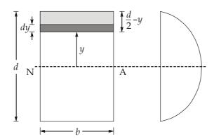
Shear stress at 'y' distance from neutral axis.
