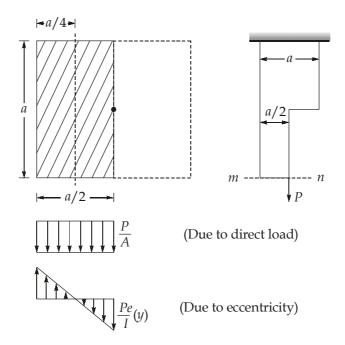
Maximum compressive stress at section mn is given by
