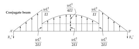
The reaction at A' and B' are equal due to symmetry.
