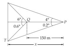
$x (\tan 4^{\circ} + \tan 0.2^{\circ}) = (x - 150) (\tan 6^{\circ} + \tan 0.6^{\circ})$   $\Rightarrow \qquad 0.0734 \ x = (x - 150) (0.11558)$   $\Rightarrow \qquad 0.04218 \ x = 17.337$   $\Rightarrow \qquad x = 411.024 \text{ m}$   $\therefore \qquad \text{Height of tower} = 411.024 (\tan 4^{\circ} + \tan 0.2^{\circ})$ = 30.176 m
