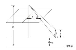
Given: H = 700 m,  $h_{avg} = 250 \text{ m}$ Relief displacement,  $d = r_1 - r$ = 112.5 - 82.40 = 30.1 mm $d = \frac{hr_1}{H - h_{avg}}$ ·.·
