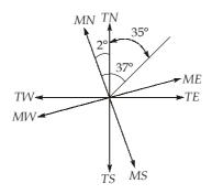
Now rate of annual magnetic declination is 5'E, so in 36 years i.e. 1985 to 2021 magnetic meridian got shifted by  $5 \times 36$  i.e. 180' means 3° in east ward side. So net declination in 2021 is 1°E.
