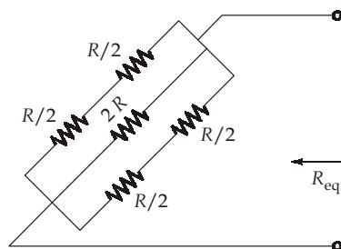
$$R_{eq} = 2R \parallel R \parallel 2R \parallel \frac{R}{2} = \frac{2R \left( \frac{R}{2} \right)}{2R + \frac{R}{2}} = \frac{R^2}{5R} \times 2$$
