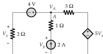
The Node voltage  $V_A = (4 + V_x)$  Volts.
