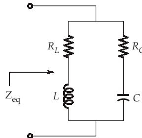
Equivalent impedance of the circuit is  $Z_{eq'}$
