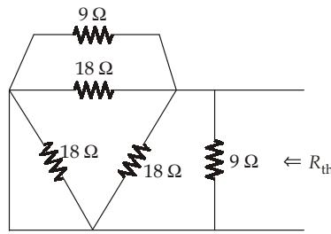
$$R_{th} = 9 \parallel [(9 \parallel 18) \parallel 18] = 9 \parallel \frac{9}{2} = \frac{9 \times \frac{9}{2}}{9 + \frac{9}{2}} = \frac{9 \times 9}{27} = 3 \Omega$$
