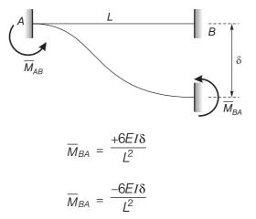
If settlement of supports causes rotation of member in clockwise direction the fixed and moment developed will be in anticlockwise direction vice-versa.
