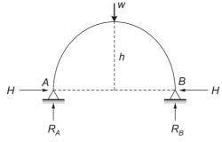
We know the horizontal thrust in two hinged parabolic arch subjected to concentrated load *W* at crown in which moment of Inertia (I) =  $I_0$  sec  $\theta$  is given by
