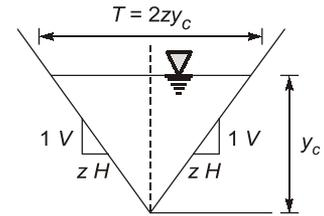
**NOTE:** Section factor ( $z$ ): It is a function of depth ' $y$ ' for a given channel geometry.
