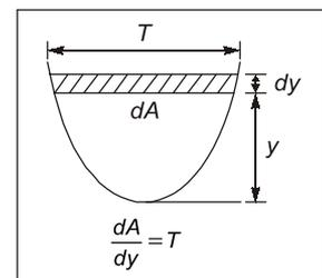
$$\frac{Q^2 T}{g A^3} = 1 \quad \text{For any channel (condition for critical state of flow)}$$
