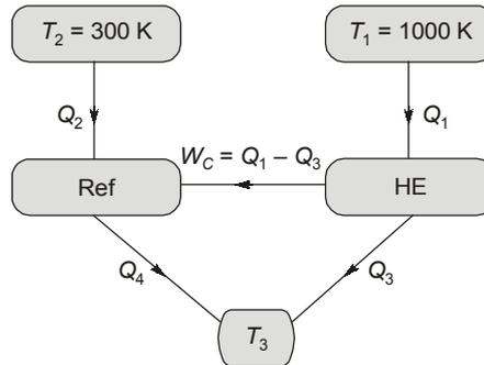
$$\Rightarrow W_c = Q_2 \left( \frac{T_3 - T_2}{T_2} \right) \quad \dots(ii)$$
