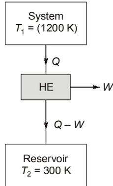
$$\text{Heat removed from the system, } Q_1 = \int_{T_1}^{T_2} C_v dT = \int_{1200}^{300} (0.05T^2) dT$$
