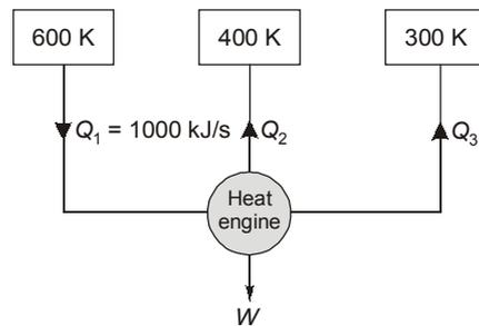
$$\begin{aligned} Q_1 &= Q_2 + Q_3 + W && \text{(As per 1<sup>st</sup> law of thermodynamics)} \\ 1000 &= Q_2 + Q_3 + 50 \\ \Rightarrow Q_2 + Q_3 &= 950 \text{ kJ/s} && \dots(i) \end{aligned}$$
