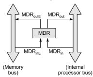
MDR is directly connected to data lines of the processor. It has 2 input and 2 output. Data may be loaded into MDR either from memory or from internal bus. Data present in MDR may be placed on either bus are memory. It requires total 4 control signals.
