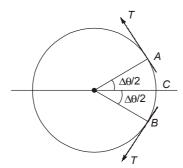
Consider a small part ACB of the ring that subtends an angle  $\Delta\theta$  at the centre. Let *T* be tension in the ring.
