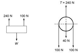
So, 240 + 100 = W (240 N includes weight of pulley and tension carried by rope) W = 340 N
