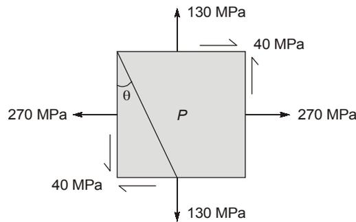
$$\begin{aligned}\sigma_{1,2} &= \frac{\sigma_x + \sigma_y}{2} \pm \frac{1}{2} \sqrt{(\sigma_x - \sigma_y)^2 + 4\tau_{xy}^2} \\ &= \frac{270 + 130}{2} \pm \frac{1}{2} \sqrt{(270 - 130)^2 + 4 \times 40^2} \\ &= 200 \pm \frac{1}{2} \sqrt{140^2 + 4 \times 1600} \\ &= 200 \pm 80.62 \text{ MPa} \\ \sigma_1 &= 280.62 \text{ MPa} \\ \sigma_2 &= 119.38 \text{ MPa}\end{aligned}$$
