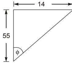
$$\text{Shear strain, } \gamma = \tan \phi = \frac{14}{55} = 0.2545$$
