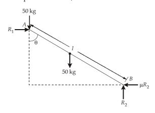
$$\Sigma F_{x} = 0 \Rightarrow R_{1} = \mu R_{2}$$
