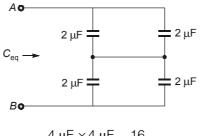
$$C'_{eq} = \frac{4 \,\mu\text{F} \times 4 \,\mu\text{F}}{8 \,\mu\text{F}} = \frac{16}{8} = 2 \,\mu\text{F}$$
