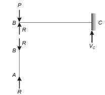
Deflection at A in beam BC = Compression in column AB
