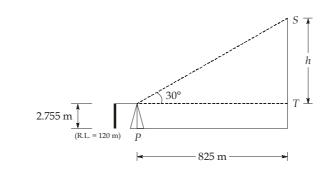
RL of top of tower = Height of instrument at P + h= (120 + 2.755) + 825 tan 30° = 599.07 m
