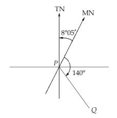
True bearing of PQ = Magnetic bearing + Magnetic declination (E) =  $140^{\circ} + 8^{\circ}05'$ =  $148^{\circ}05'$
