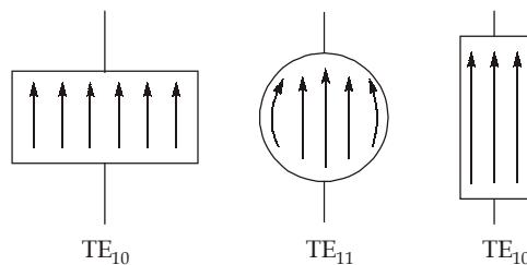
Due to change in orientation of the guide, the field orientation does not change, but ' $a$ ' becomes smaller dimension than ' $b$ '. As the field orientation doesn't change,  $\text{TE}_{10}$  mode is excited in the waveguide.
