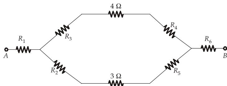
$$R_1 = R_6 = \frac{4.5 \times 7.5}{4.5 + 7.5 + 3} = 2.25 \Omega$$
