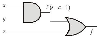
**Step 1:** To propagate the fault at output, i.e.,  $f = P$ ,
