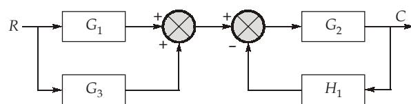
The block diagram can further be simplified as below:
