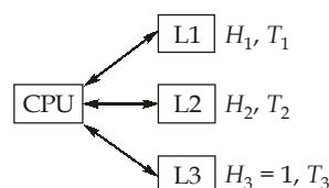
$$\text{AMAT} = H_1 T_1 + (1 - H_1) H_2 T_2 + (1 - H_1)(1 - H_2) T_3$$
