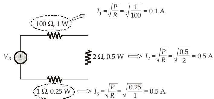
Thus, for safe operation current  $I = \min \{0.1 \text{ A}, 0.5 \text{ A}, 0.5 \text{ A}\} = 0.1 \text{ A}$
