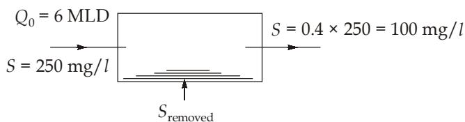
$$\begin{aligned}\text{Suspended solids removed} &= (250 - 100) \frac{\text{mg}}{\text{l}} \times 6 \times 10^6 \frac{\text{l}}{\text{d}} \\ &= 900 \text{ kg/d}\end{aligned}$$
