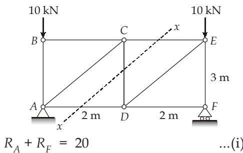
$$R_A + R_F = 20 \quad \dots(i)$$
