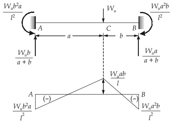
$$BM_{\max-B} = \frac{W_u a^2 b}{l^2} \text{ (at } B\text{)}$$
