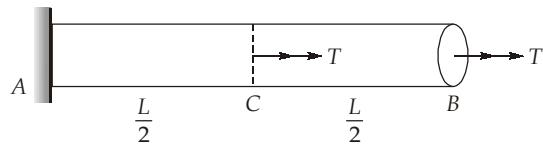
$$\therefore \text{Torque in the part } AC = 2T$$
