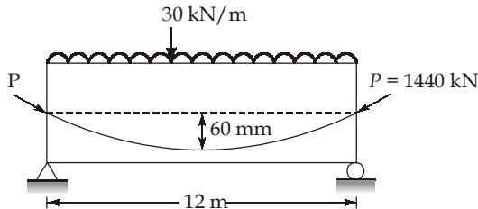
Intensity of equivalent load due to parabolic cable.
