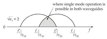
$\therefore$  The range of dielectric constant required for single mode operation in both the rectangular waveguides is  $\sqrt{\epsilon_r} < 2$  i.e.,  $\epsilon_r < 4$ .
