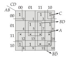
In the 4-variable K-map shown above, there are two octet and two quads. The simplified expression is given by,
