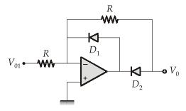
During –ve half cycle of  $V_{\it o1^{\prime}}$   $D_1$  is ON and  $D_2$  is OFF.
