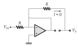
Therefore,  $V_o = 0$  in the –ve half cycle of  $V_{o1}$ .
