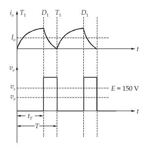
The expression for average dc machine output current is based on continuous armature inductance current. Therefore, the switching period must be shorter than the time  $t_x$ , given by below expression, for the current to reach zero, before the next switch on-period. That is  $t_x = T$  and  $\alpha = 0.30$ .
