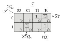
$$T = \overline{X}Y + Y\overline{Q}_n + X\overline{Y}Q_n$$
