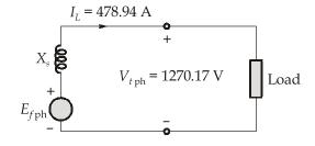
$$\left| E_{f \, \text{ph}} \right| = \sqrt{\left( V_{tph} \cos \theta + I_a R_a \right)^2 + \left( V_{tph} \sin \theta + I_a X_s \right)^2}$$
