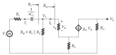
Let the resistance  $R_B = R_1 \parallel R_2$
