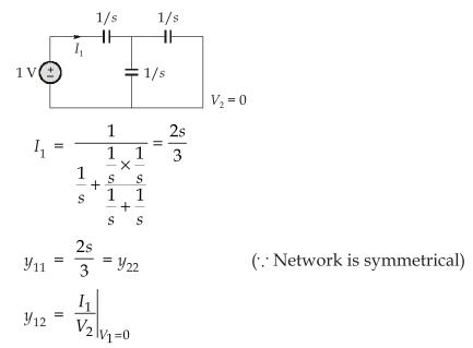
Considering  $V_1$  = 0, the circuit can be drawn as below.
