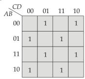
$$P = \overline{A}\overline{B}\overline{C}D + \overline{A}\overline{B}C\overline{D} + \overline{A}B\overline{C}\overline{D} + \overline{A}BCD + A\overline{B}\overline{C}\overline{D} + A\overline{B}CD + AB\overline{C}D + ABC\overline{D}$$
