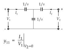
Considering  $V_2$  = 0, the circuit can be drawn as below.
