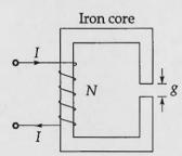
Length of iron path = 120 cm, g = 0.5 cm, area of cross-section of iron =  $5 \times 5$  cm<sup>2</sup>,  $\mu_r = 1500$ , I = 2 A, N = 1000 turns.
