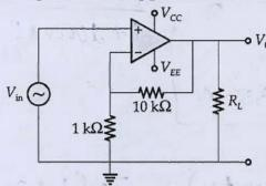
A=20000,  $R_i=2$  M $\Omega$ ,  $R_0=75$   $\Omega$ ,  $f_0=5$  Hz, supply voltage =  $\pm 15$  V, output voltage swing =  $\pm 13$  V. Identity the circuit.
