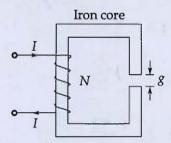
Length of iron path = 120 cm, g = 0.5 cm, area of cross-section of iron =  $5 \times 5$  cm<sup>2</sup>,  $\mu_r = 1500$ , I = 2 A, N = 1000 turns.
