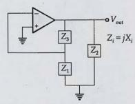
The op-amp in the circuit has a finite open loop gain  $(A_v)$ , finite output resistance  $(R_0 > 0)$  and it is ideal in all other aspects.  $Z_1$ ,  $Z_2$  and  $Z_3$  are purely reactive elements with magnitudes  $|X_1|$ ,  $|X_2|$  and  $|X_3|$ . Prove that  $X_1$  and  $X_2$  must be of the same type of reactance (i.e., both must be either capacitive or inductive) to produce sustained oscillations.
