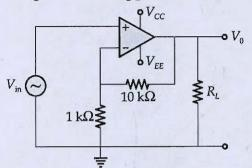
A = 20000,  $R_i = 2$  M $\Omega$ ,  $R_0 = 75$   $\Omega$ ,  $f_0 = 5$  Hz, supply voltage =  $\pm 15$  V, output voltage swing =  $\pm 13$  V. Identity the circuit.
