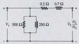
The load impedance connected to the high-tension terminals is  $380 + j230 \Omega$ . For a primary voltage of 250 V,
