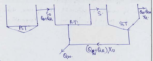
(I) Volume:  $\frac{Q_0(50-5)Q_CY}{(1+k_0Q_C)X}$  >  $\frac{150-5)mq \times 10A \times 0.5}{(1+0.05 \times 10) \times 3000 \text{ ma}}$
