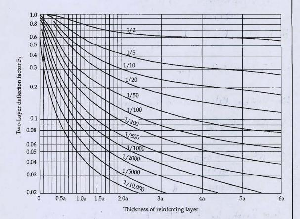
Design the pavement section for 4100 kg wheel load with tyre pressure of  $5 \, \text{kg/cm}^2$  for an allowable deflection of 0.5 cm using Burmister's approach.
