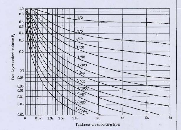
Design the pavement section for  $4100 \, \text{kg}$  wheel load with tyre pressure of  $5 \, \text{kg/cm}^2$  for an allowable deflection of  $0.5 \, \text{cm}$  using Burmister's approach.
