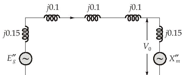
$$\begin{aligned} E_g'' &= V_0 + I_{pu}(X_{T1} + V_{T2} + X_L + X_g'') \\ &= 0.963\angle 0^\circ + 0.778\angle 36.86 (j0.1 + j0.1 + j0.1 + j0.15) \\ &= 0.8034\angle 20.41^\circ \end{aligned}$$
