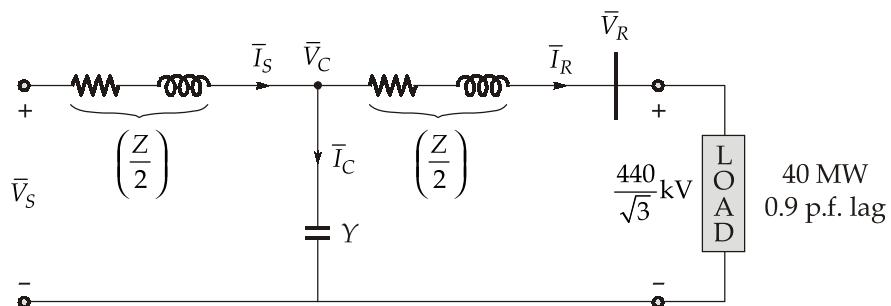
$$\begin{aligned} \text{Node voltage, } \bar{V}_C &= \bar{V}_R + \bar{I}_R \left( \frac{Z}{2} \right) \\ &= 127 \times 10^3 \angle 0^\circ + (116.62 \angle -25.84^\circ) \left( \frac{134.16}{2} \angle 63.43^\circ \right) \end{aligned}$$
