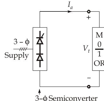
$$\begin{aligned}V_t &= E_b + I_{a_1} R_a \\ 461.081 &= K_m \times \frac{2\pi \times N_1}{60} + I_{a_1} \times 1 \\ &= 3.374 \times \frac{2\pi \times 1200}{60} + I_{a_1}\end{aligned}$$
