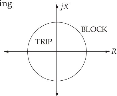
$$|Z_l|^2 = R_l^2 + X_l^2 \quad \dots(\text{equation of circle})$$
