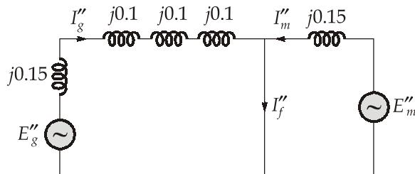
$$\begin{aligned} I_0'' &= \frac{E_g''}{j0.15 + j0.1 + j0.1 + j0.1} \\ &= \frac{0.8034\angle 20.41^\circ}{0.45\angle 90^\circ} = 1.785\angle -69.59^\circ \text{ p.u.} \end{aligned}$$
