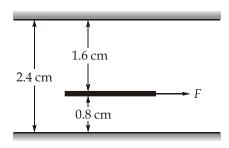
:. Shear force on the upper side of the thin plate,
