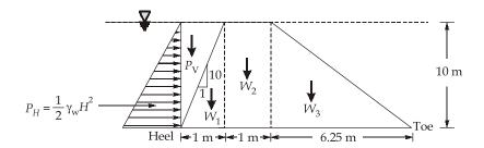
All the forces will be calculated by considering unit length of masonry dam. Let W be the self weight of the masonry dam,  $P_H$  be the horizontal force due to water and  $P_V$  be the vertical force due to triangular block of water. Neglecting uplift forces, we calculate the respective parameters as tabulated below:
