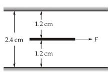
Case I: When the thin plate is in the middle of the two plane surfaces [Refer to Figure]
