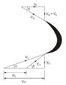
2. The wheel vane angle at inlet *i.e.*  $\theta$
