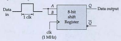
Draw and calculate the output and delay provided by the above shift register in clear steps.
