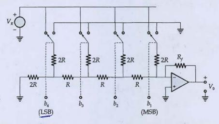
Assume the feedback resistance  $R_f$  of the op-amp is variable, the resistance  $R=5~\mathrm{k}\Omega$  and  $V_R=10~\mathrm{V}$ . Determine the value of  $R_f$  that should be connected to achieve the following output conditions:
