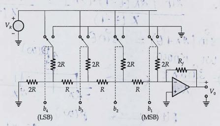
Assume the feedback resistance  $R_f$  of the op-amp is variable, the resistance  $R=5~\mathrm{k}\Omega$  and  $V_R = 10 \text{ V}$ . Determine the value of  $R_f$  that should be connected to achieve the following output conditions:
