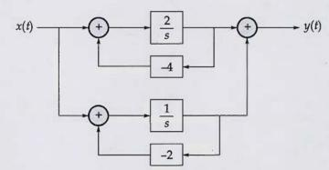
Determine a differential equation relating the input x(t) to the output y(t) of this system.
