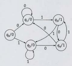
Get the excitation equations and Boolean equations for output Z of Mealy machine. Also design the Mealy machine using J-K flip-flop.
