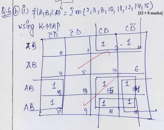
$$\frac{7 - BC + AC + AD}{\overline{F} = BC + AC + AD} = \overline{BC \cdot AC \cdot AD}$$
