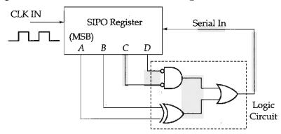
Explain its operation by drawing waveforms for the output of shift register (ABCD). Assume that initially shift register is in state ABCD = 1111.
