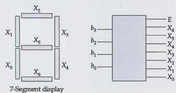
where, E = 0 for valid digit with the display showing the corresponding digit.
