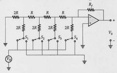
Determine the values of  $R_f$  that should be connected to achieve the following output conditions:
