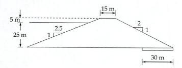
Also determine the seepage discharge per unit length if the coefficient of permeability is 40 m/day.
