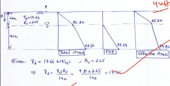
$$7_{sub} = \frac{3\omega(6_{s}-1)}{1+e} = \frac{10.997 \text{ kN/m}^{3}}{1}$$
