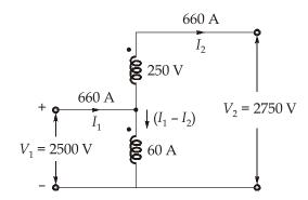
For two winding transformer primary rated current,
