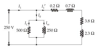
Therefore, total series impedance is  $4 + j3 = 5 \angle 36.9^{\circ}$
