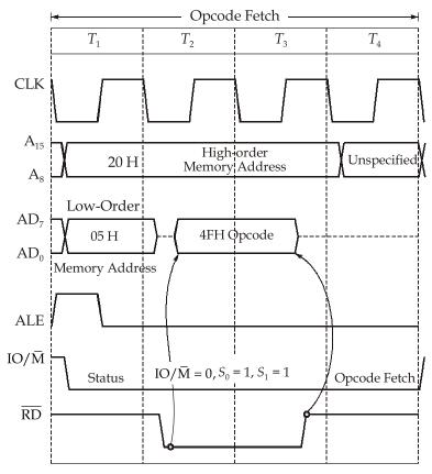
• The byte is placed in the instruction decoder of the microprocessor and the task is carried out according to the instruction. The machine code or the byte (4FH) is decoded by the instruction decoder, and the contents of the accumulator are copied into register C. This task is performed during the period  $T_4$ .
