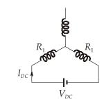
$$R_1 = \frac{V_{DC}}{2I_{DC}} = \frac{13.6}{2 \times 28} = 0.2428 \text{ A}$$
