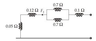
From the positive-sequence network, the equivalent impedance upto the point of the fault is given by
