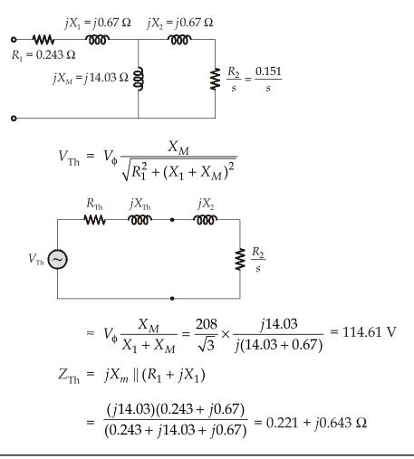
$$S_{\text{max}} = \frac{R_2}{\sqrt{R_{\text{Th}}^2 + (X_{\text{Th}} + X_2)^2}} = \frac{0.151}{\sqrt{(0.243)^2 + (0.643 + 0.67)^2}}$$
