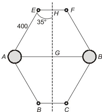
**Q.22** In porter governor for the controlling force diagram shown below, the mass of each ball is 5 kg, the controlling force is \_\_\_\_\_ Newton.
