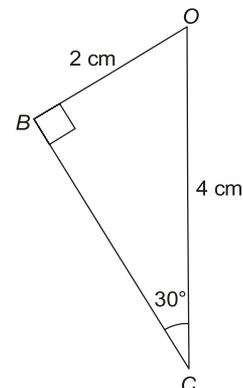
At this position  $\angle OBC$  will be  $90^\circ$ , velocity of B perpendicular to CD will be zero hence  $\omega_{CD} = 0$ . So, Coriolis acceleration will be zero.
