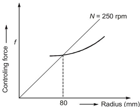
**Q.23** The controlling force  $F$  in Newton and  $r$  the radius of rotation in mm for a spring loaded governor are related by the expression
