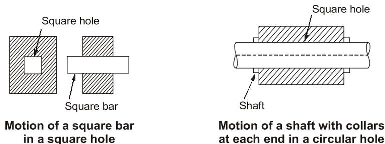
e.g. piston and cylinder (in a steam engine) form a pair. Motion of the piston is limited to a definite direction (i.e. it will only reciprocate) relative to the cylinder irrespective of the direction of motion of the crank.
