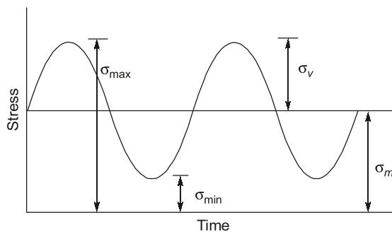
**A typical stress cycle showing maximum, mean and variable stresses**
