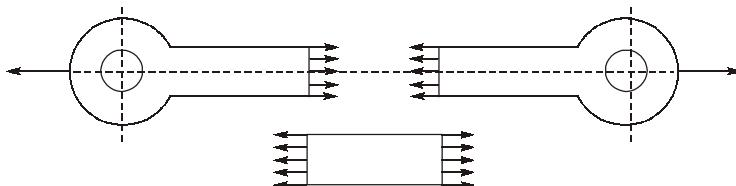
Stresses developed in a link subjected to uniaxial loading
