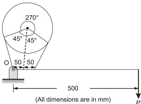
Find, the minimum force (in N) for its direction required at the end of the brake lever to stop the drum, if 50 kW power is to be absorbed
