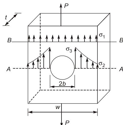
Stress concentration due to a central hole in a plate subjected to an uni-axial loading.
