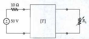
The output port is connected to a variable load for maximum power transfer. Find  $R_L$ and the maximum power transferred.
