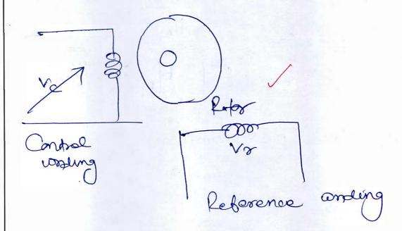
Ac Seavomoter as a 2-phase mourteen troter. The Control phase winding is variable.
