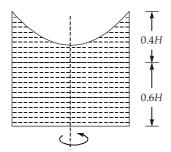
Given pressure at centre at bottom =0.6H m of liquid.
