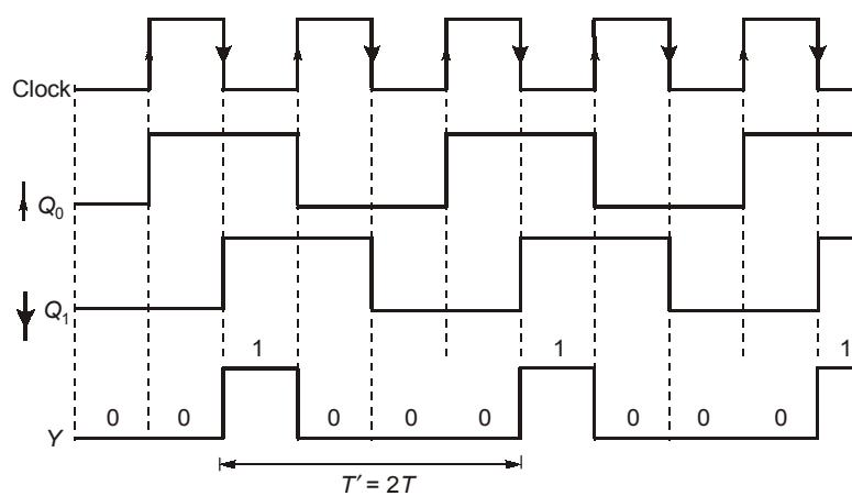
$$\begin{aligned} \text{Duty cycle} &= \frac{T_{ON}}{T_{ON} + T_{OFF}} \times 100\% = \frac{1}{1+3} \times 100\% \\ &= \frac{1}{4} \times 100\% = 25\% \end{aligned}$$
