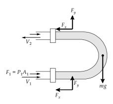
$$-F_x + (P_1 - P_a) \times A_1 + (P_2 - P_a) \times A_2 = m_2 V_2 - m_1 V_1$$
