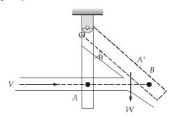
Force on an inclined stationary plate in normal direction to the plate,
