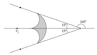
For theoretical force it is assumed that velocity is not reduced as water passes around each cup,
