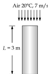
The flow is along 3 m side of the plate, and thus the characteristic length is  $L = 3$  m. Both sides are exposed to air flow,
