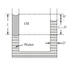
$$L = \frac{V_{oil} \times 4}{\pi D^2} = \frac{3.25 \times 10^3 \times 4}{\pi \times 6.35^2} = 102.623 \text{ mm}$$
