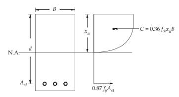
Compressive force in beam section is given as,
