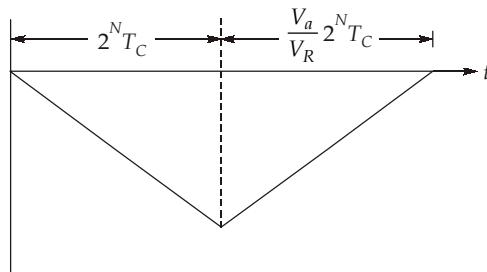
$$\text{Total conversion time, } (t) = 2^N T_C + \frac{V_a}{V_R} \cdot 2^N T_C$$
