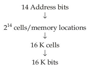
Since 16 K cells provide a capacity of 16 Kbits, so cell size must be 1 bit.
