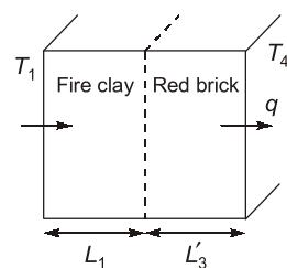
$$q = \frac{T_1 - T_4}{\frac{L_1}{k_1 A} + \frac{L_2}{k_2 A} + \frac{L_3}{k_3 A}} ; \quad q = \frac{T_1 - T_4}{\frac{L_1}{k_1 A} + \frac{L'_3}{k_2 A}}$$
