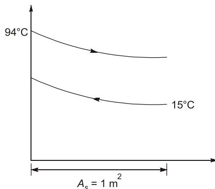
$$NTU = \frac{UA_s}{C_{\min}} = \frac{1075 \times 1}{305.4} = 3.52$$
