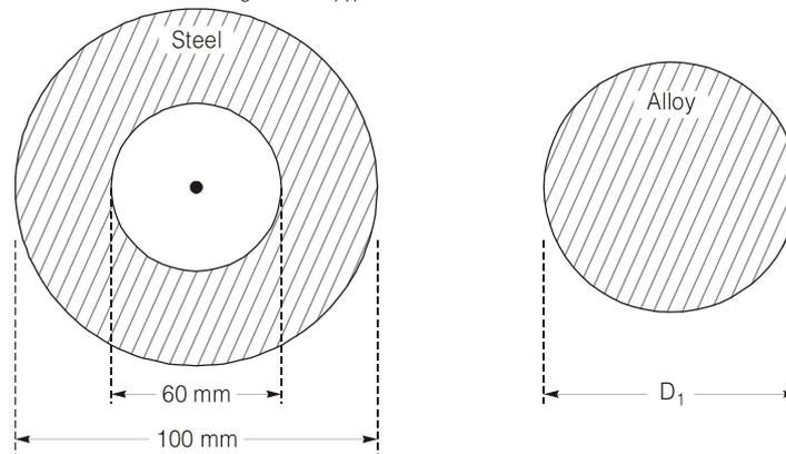
$$(Z_P)_{\text{Hollow shaft}} = \frac{J_{\text{Hollow}}}{D/2} = \frac{\pi (D^4 - d^4)}{16 D}$$
