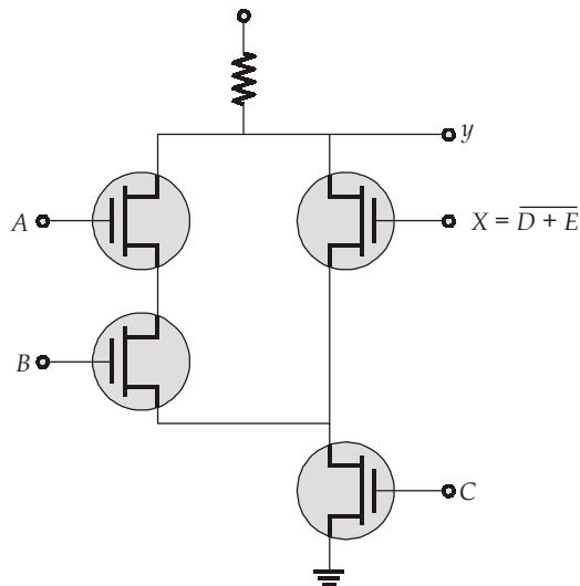
$$\therefore y = \overline{(AB + X) \cdot \bar{C}} = \overline{(AB + (D + E)) \cdot C}$$
