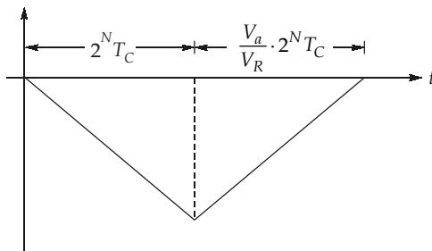
$$\text{Total conversion time, } (t) = 2^N T_C + \frac{V_a}{V_R} \cdot 2^N T_C$$
