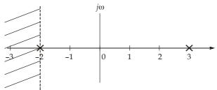
Also, ROC doesn't consists of  $j\omega$  axis, therefore, system is unstable.
